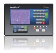
**InteliGen**® is a comprehensive controller for both single and multiple gen-sets operating in standby or parallel modes.
